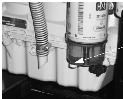
Drain for water separator bowl for engines so equipped
